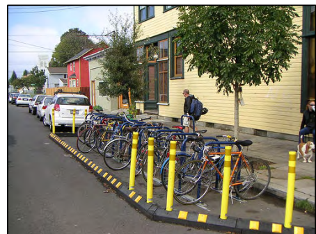
On-street automobile parking (shown here in Portland, OR) can easily and inexpensively be converted to on-street bicycle parking.
