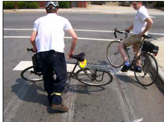
Testing the sensitivity of a loop detector
